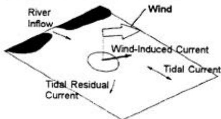
As for drift phenomenon, processes such as tidal current, tidal residual current, river inflow, and wind-induced current are modeled. Data base of tidal current with a mesh unit of 1 km has been prepared in this model. Statistical data of marine wind are provided in the model, however, the utilization of weather forecast data is preferable to improve the accuracy of prediction in an oil spill.
