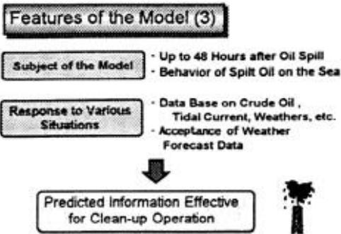
The model can predict the behavior of spilt oil on the sea in a period up to 48 hr after spillage. The model contains basic data including properties of crude oil and petroleum products, and tidal currents in the target area of sea, and predicts with enough accuracy to be effective for the clean-up operation.
