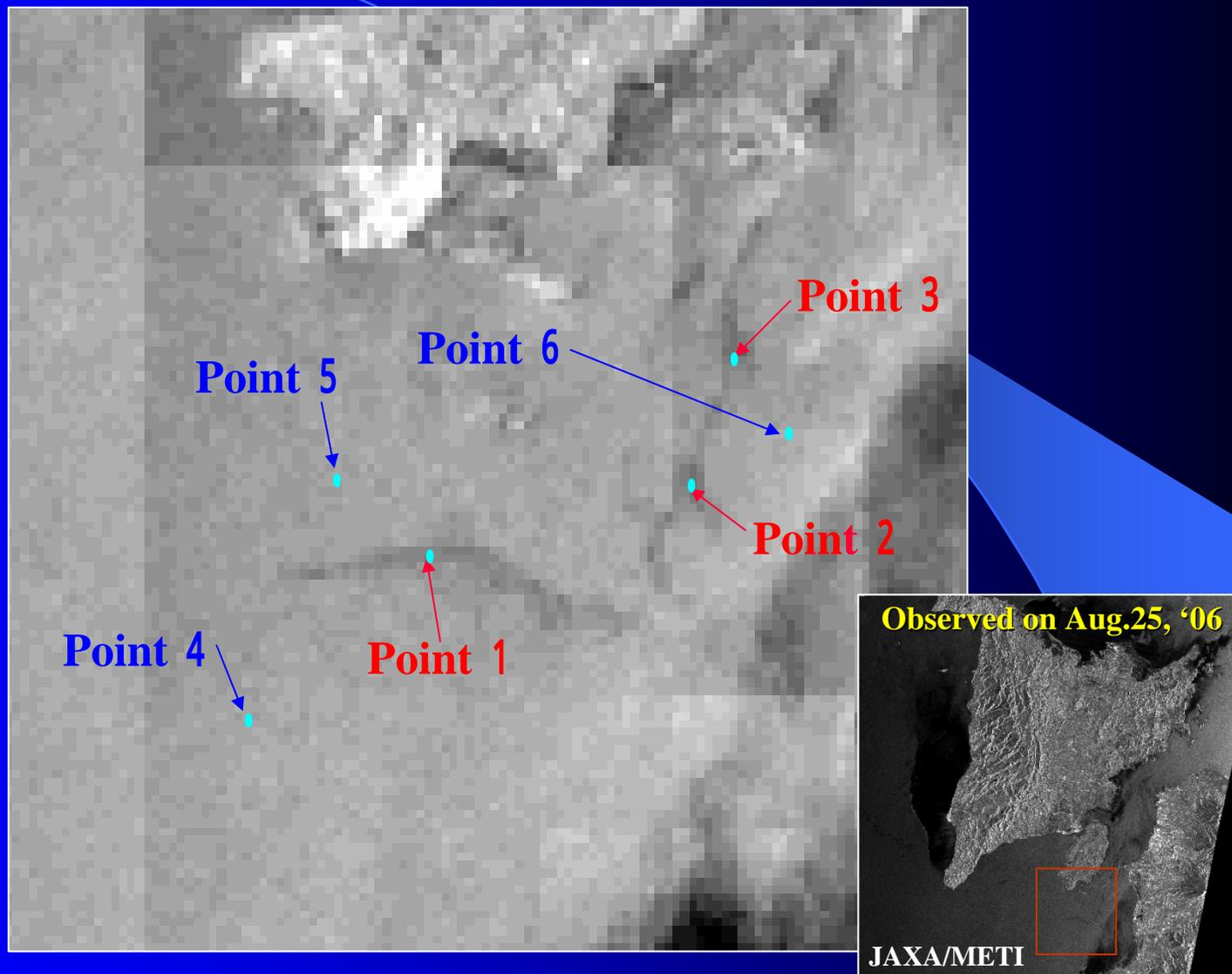
The sampling points are selected in the area detected as an spilled area : Point 1 ~ 3
