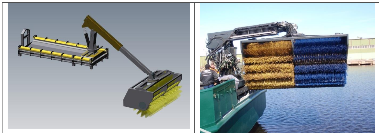
Figure 6. Design picture (left) and manufactured prototype unit prior the open water tests. L = 4000\text{mm} and D = 2000\text{ mm} .
