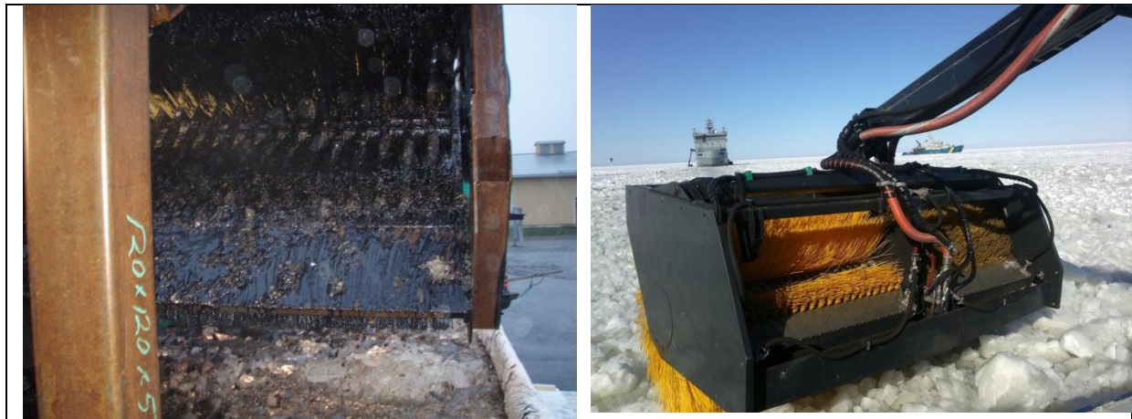
Figure 7. (Left) 4000 mm long prototype in out-door laboratory tests and (Right) oil recovery brush (L 4000 mm, D 2000 mm) in full scale offshore exercise.
