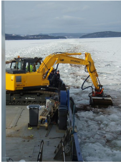
Figure 2. Oil recovery bucket connected to hydraulic excavator. Tests in 2009 in ice.(Photo: J. Pirttijärvi)
