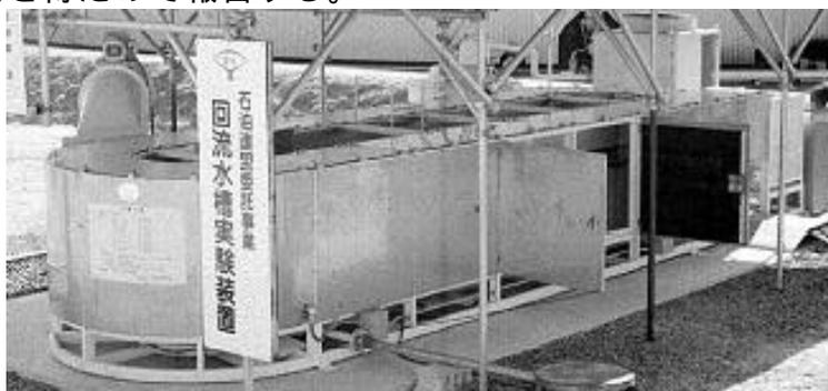
Figure 1 Circulating water channel
