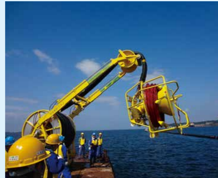
大型油回収機の投入(5号北海道基地) Use of Large Skimmer (No.5 Hokkaido Base)
