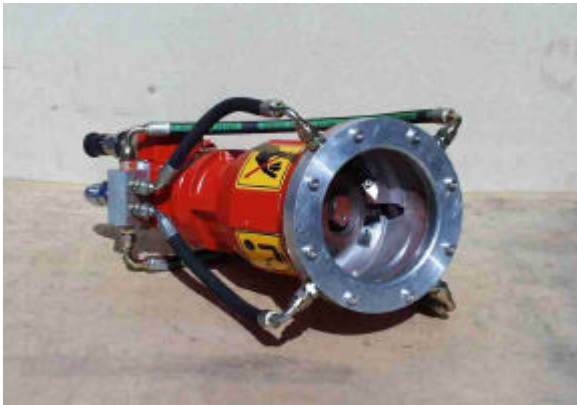
Figure 8 DOP Pump with FlemingCo Inlet Side Steam/Hot Water Injection System
