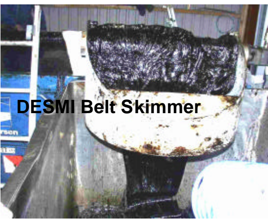
Figure 2 Mechanical Feeder Skimmers, which Have Been Tank Tested on Bitumen
