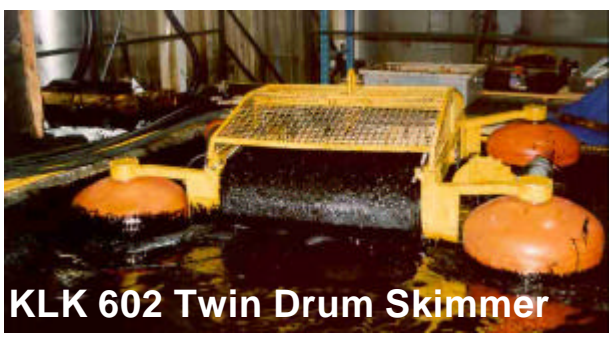
Figure 2 Mechanical Feeder Skimmers, which Have Been Tank Tested on Bitumen
